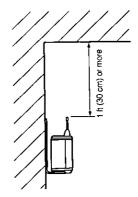
Mount the mounting bracket(provided) on the wall with 2 screws or 4 screws.
